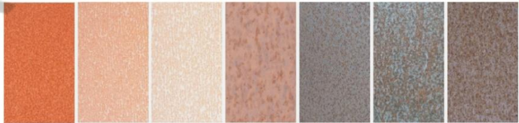
Fig. 2.3: Example of possible oxide layer appearances developed under different exposure conditions
